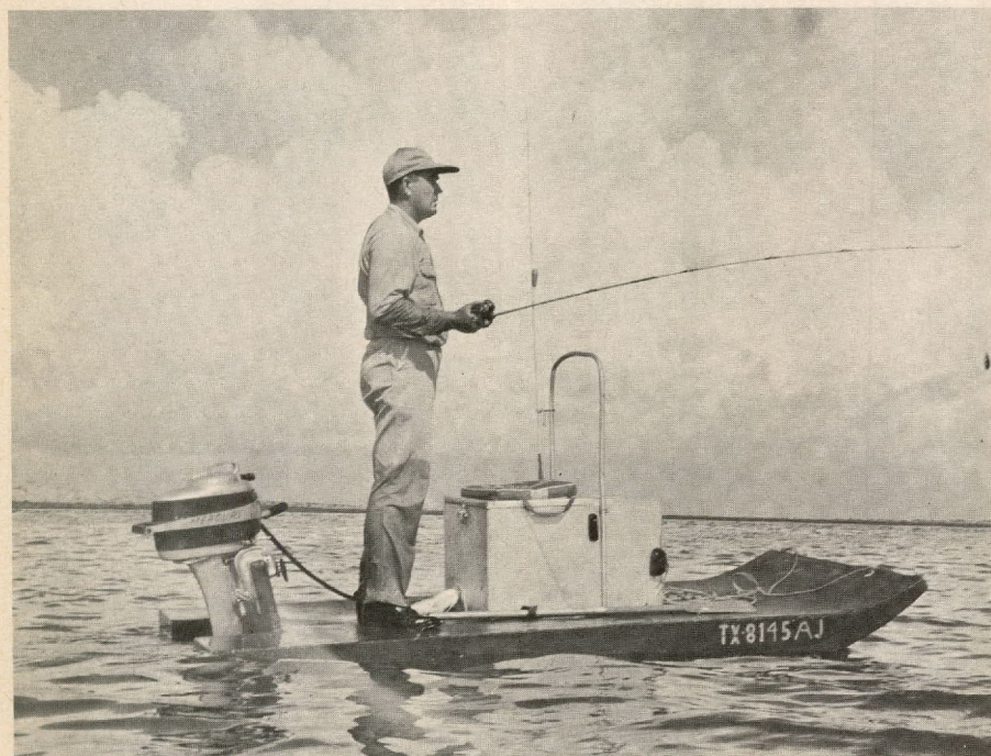
The box on standard model is used for food and ice storage as well as a seat and an observation platform. Boat can be steered by leaning from side to side.
