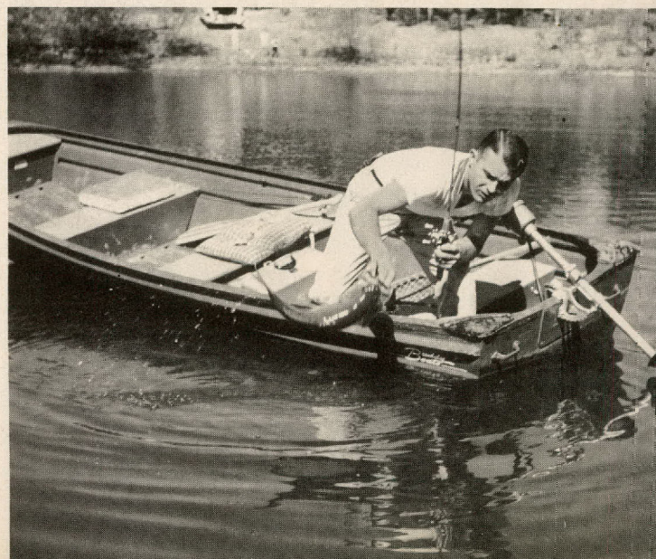
The Electra Pal is adjusted so the prop clears moss. It can be raised completely when using a gas motor for long maneuvers.
