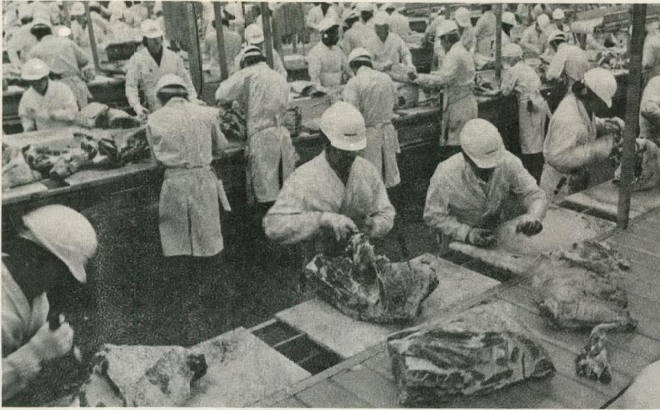
Moving conveyors transfer primal cuts of beef for fabrication, at Iowa Beef Processor's Amarillo facility. The modern plant can process up to 20,000 cattle per week when in full operation.
