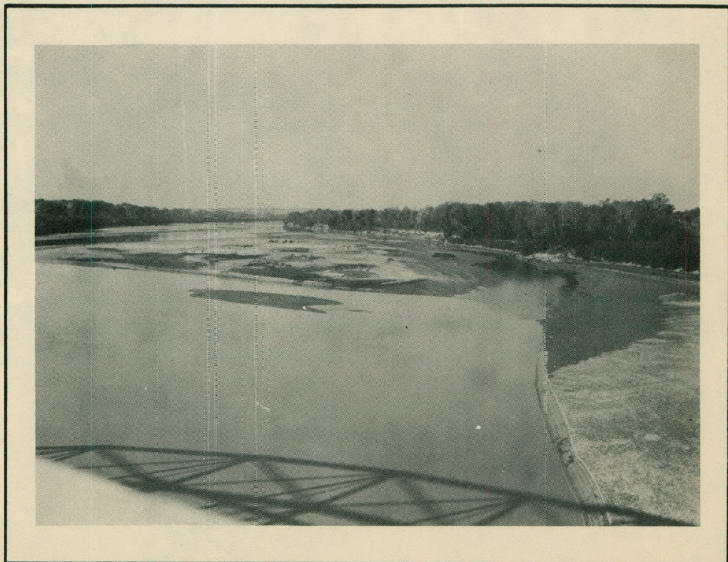
Looking upstream from silt sampling station. The stream channel is wide and sandy. There is considerable shifting of the main stream through the sandy channel. The Denison Dam is being constructed several miles upstream and at horizon in center of picture.
