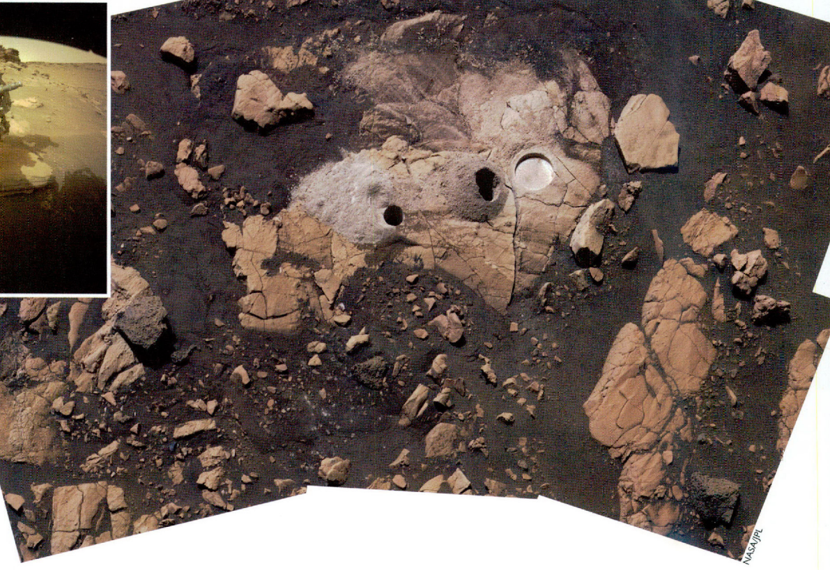
A close-up (right) shows three holes that Perseverance drilled into the rocks to analyze their composition. Top: The rover's robotic arm, which contains the drilling tools, hovers over another rock formation.
