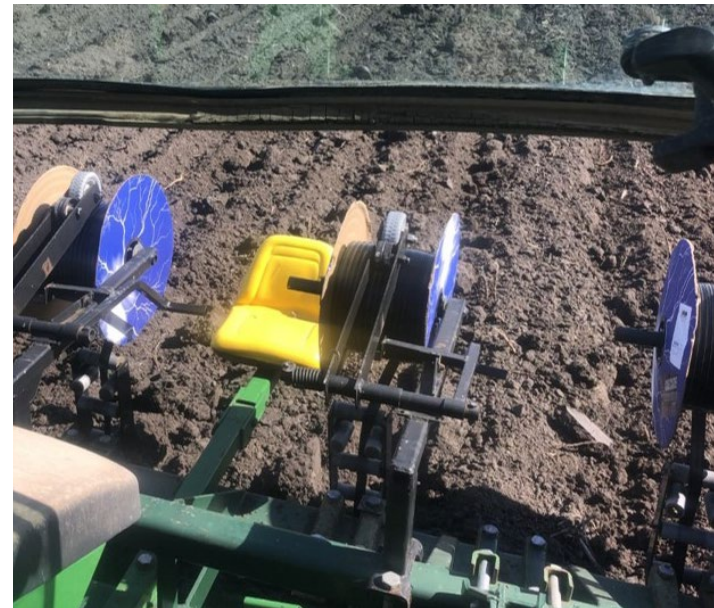
Installation of subsurface drip irrigation lines in a crop field.
