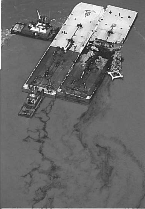
The Buffalo Marine Service barge broke in the middle, leaking oil into the channel.
