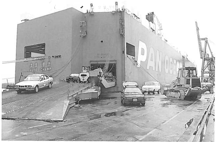
A roll-on, roll-off ship, commonly referred to as a RO/RO, drops its cargo of automobiles at the Port of Houston. RO/ROs are one of several types of specialized ships that make marine commerce possible.
