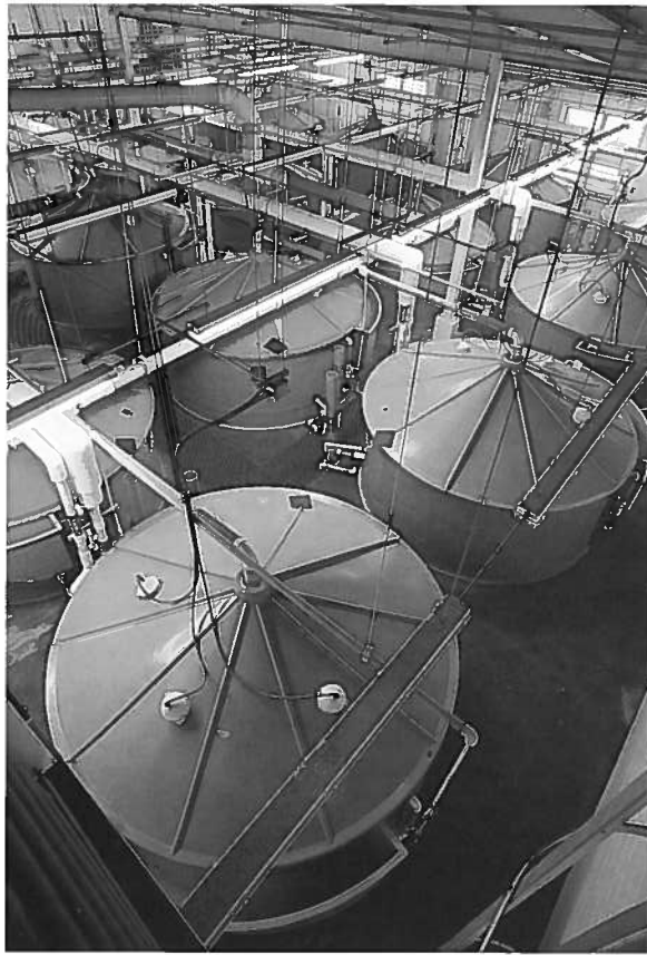
Each of these 3,500 gallon tanks at Sea Center Texas holds adult redfish or trout that produce the young fish that are restocked into the state's bay systems.
