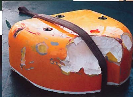
The MAX Rover remotely operated vehicle, or ROV (upper left), was tasked with performing the vast majority of artifact retrieval. The excavation had to be scaled back significantly after the MAX Rover was accidentally pulled into the propeller blades (like those pictured top right) of the SSV Carolyn Chouest. The only remnants of the ROV were a mauled piece of Styrofoam (above) and a sliced umbilical cord (left).
