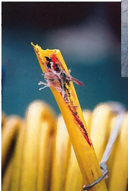
The MAX Rover remotely operated vehicle, or ROV (upper left), was tasked with performing the vast majority of artifact retrieval. The excavation had to be scaled back significantly after the MAX Rover was accidentally pulled into the propeller blades (like those pictured top right) of the SSV Carolyn Chouest. The only remnants of the ROV were a mauled piece of Styrofoam (above) and a sliced umbilical cord (left).
