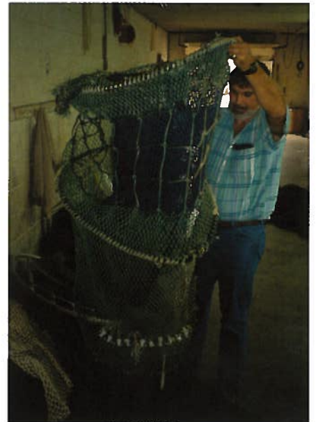
Gary Graham inspects an expanded mesh fish excluder prior to BRD testing.
