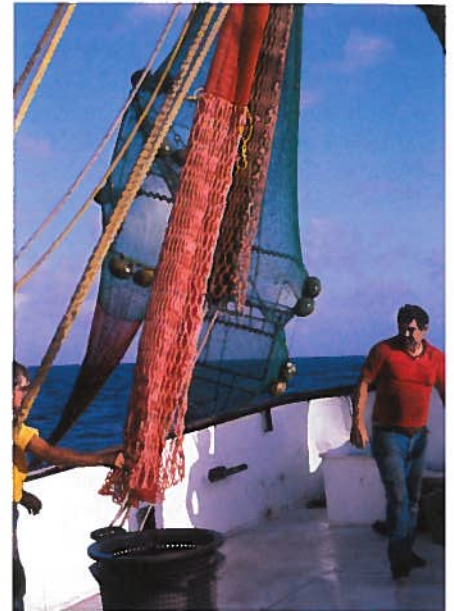
Gary Graham ducks away from a NMFS TED being pulled aboard a shrimp boat during trials in 1983.
