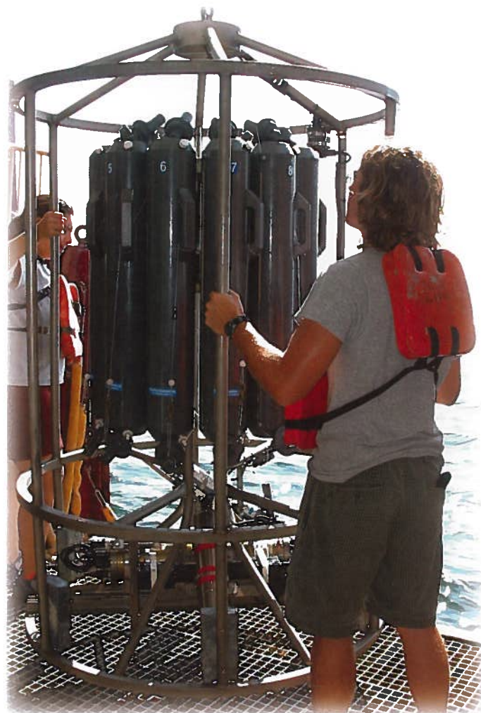
TAMU graduate students Laura Rubiano-Gomez and Keith Dupuis prepare to deploy the CTD/Rosette System, which provides data about conductivity, temperature and water depth or pressure and includes water sample collecting bottles and a dissolved oxygen sensor.
