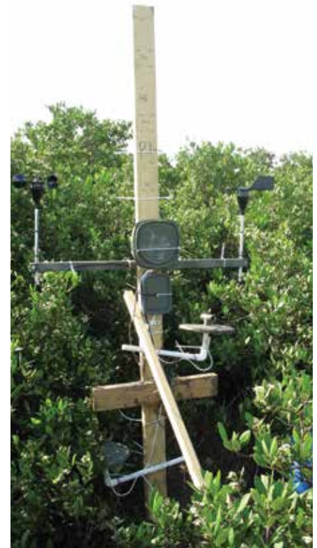
Weather stations installed in each plot measure wind speed and direction, and the temperatures of the air and soil.
