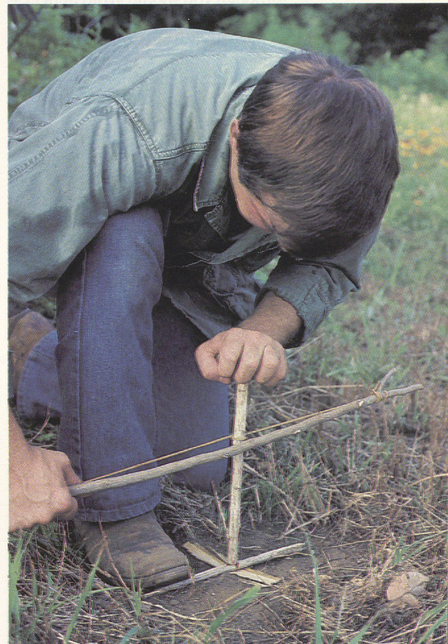
Bowdrills are primitive fire-making tools easily made from common materials such as a willow branch and a shoestring.
