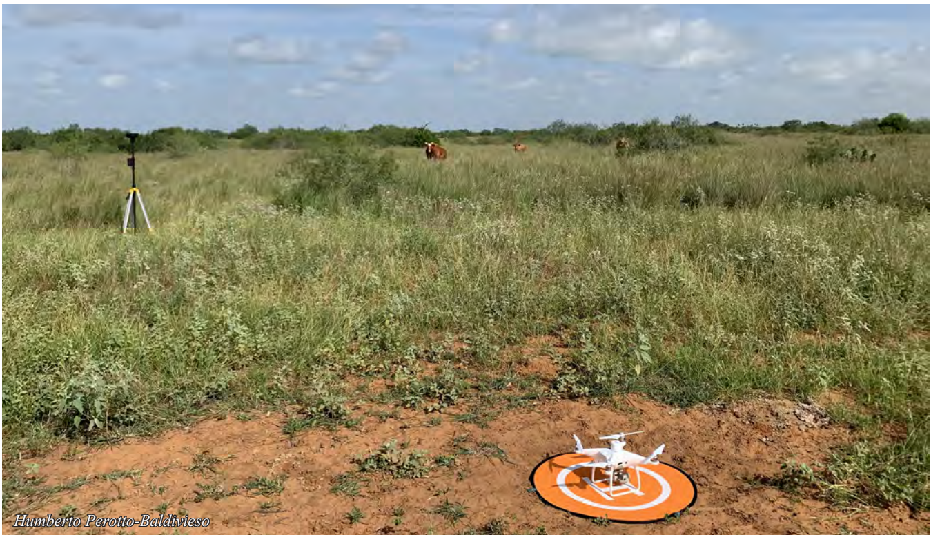
DJI Phantom 4 RTK drone used to collect imagery of vegetation in Duval County, Texas.
