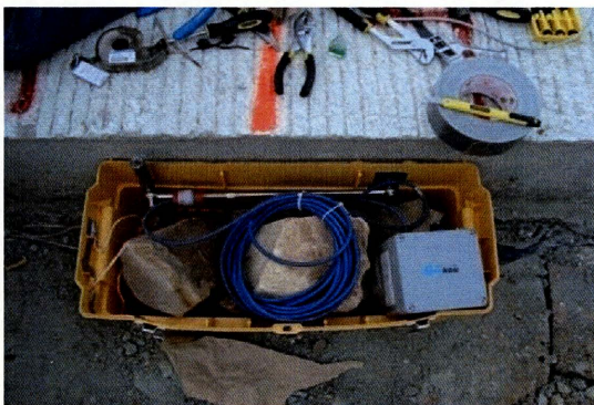
Figure 4.26 Setup of the datalogger and the crackmeter
