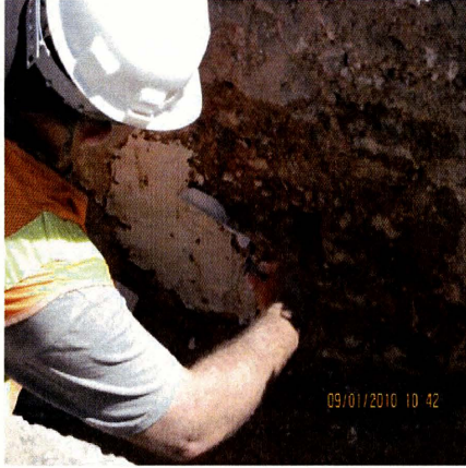
Figure 4.9 Applying plaster of Paris for good contact between pressure cell and soil
