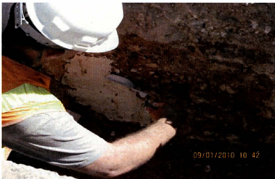
Figure 4.48 Plaster of Paris applied for the good contact between pressure cell and the soil
