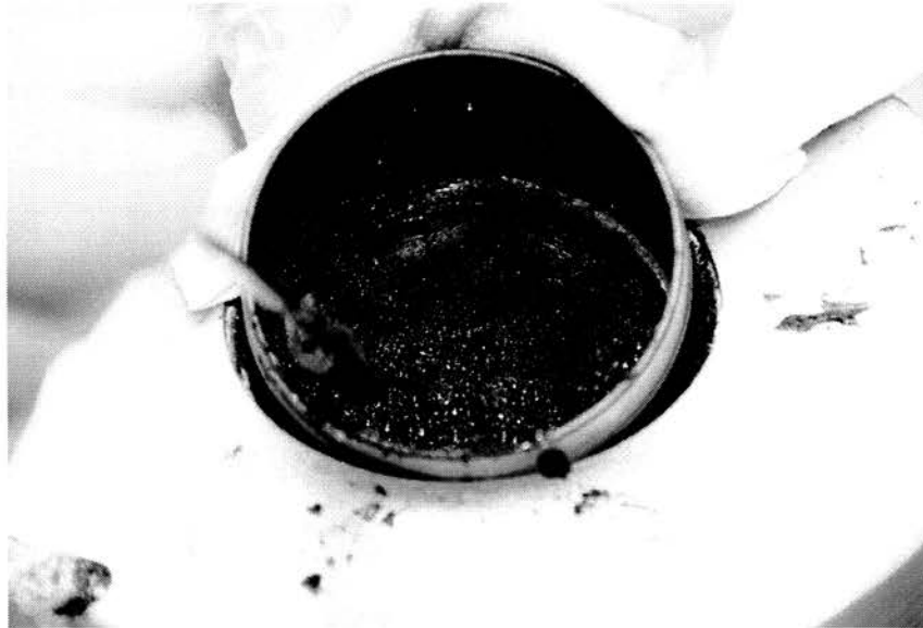
Figure 3.4. Manually mixing glass beads with the asphalt binder to prepare a homogenous mixture
