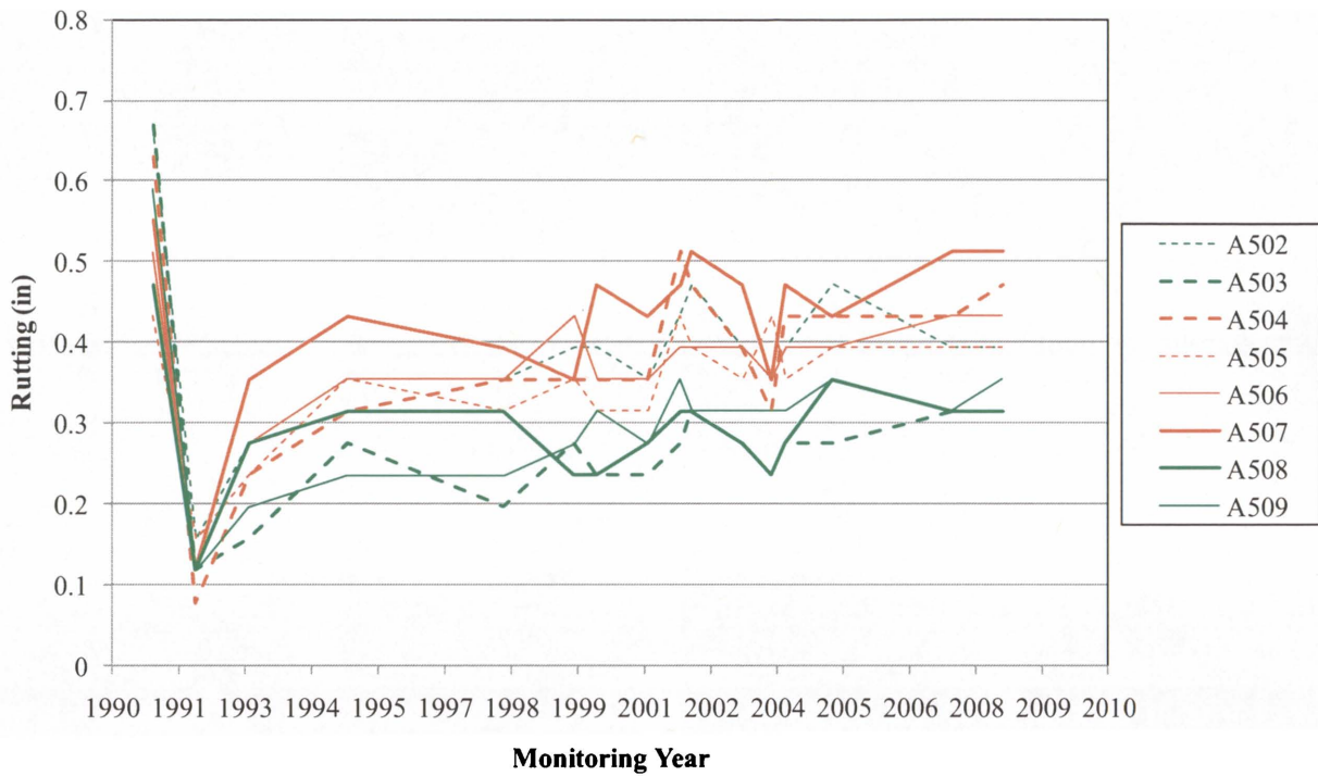
Figure 4.2: Rutting of Texas SPS-5 pavement structures
