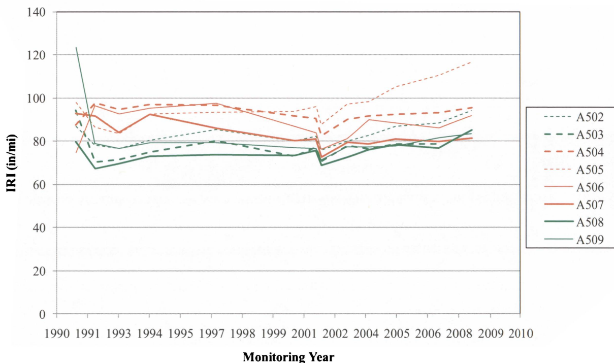
Figure 4.6: Roughness of Texas SPS-5 pavement structures
