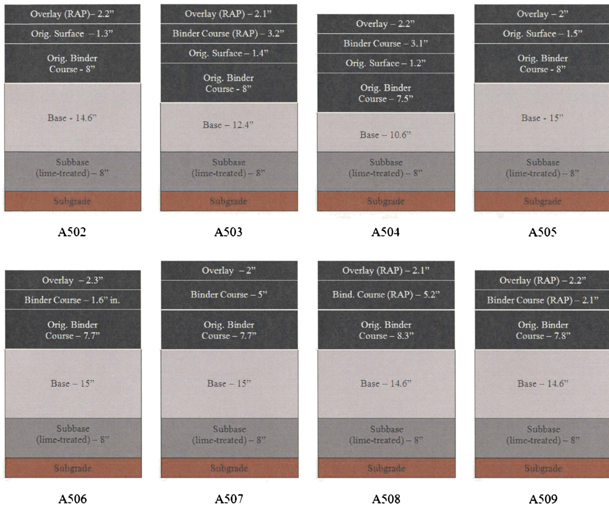
Figure 4.1: Texas SPS-5 pavement structures
