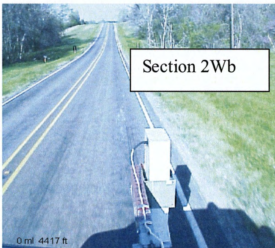
Figure C-7. GPR Survey of FM 2 (West Bound Stations 185+00 ~ 167+00).
