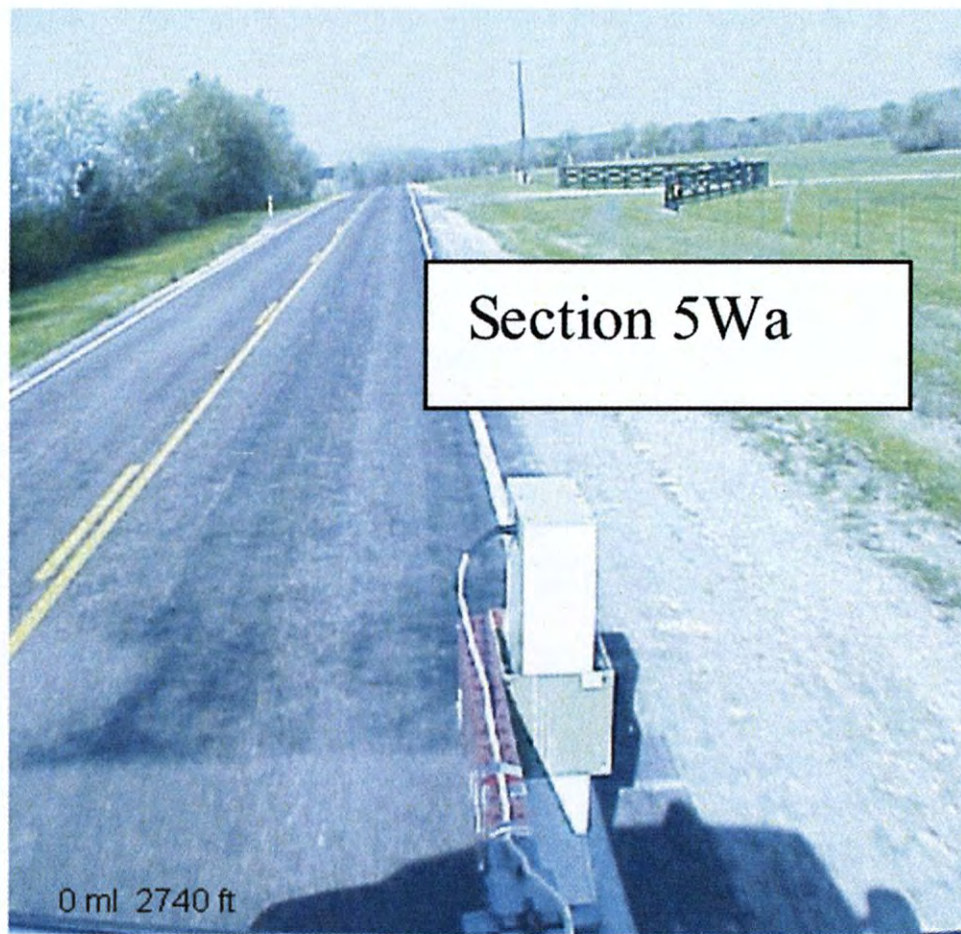
Figure C-6. GPR Survey of FM 2 (West Bound Stations 203+00 ~ 185+00).
