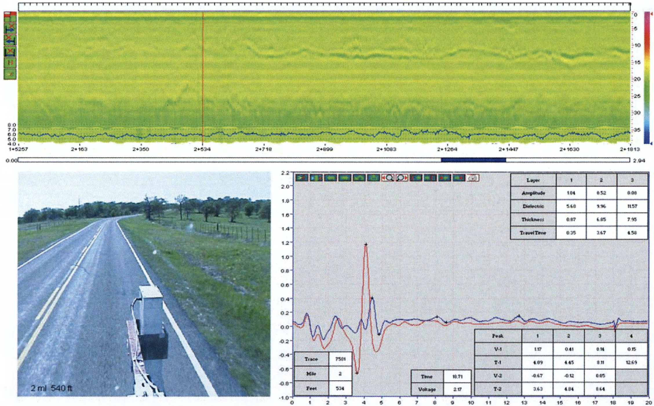
Figure C-3. GPR Data on Section 3 (Geogrid) of FM 1915.
