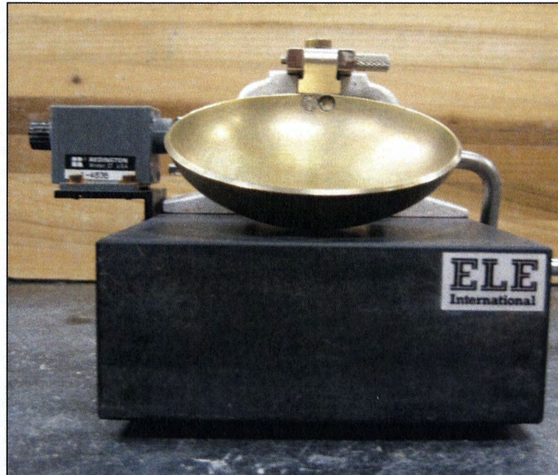
Figure A.3. Hand-Operated Liquid Limit Device.
