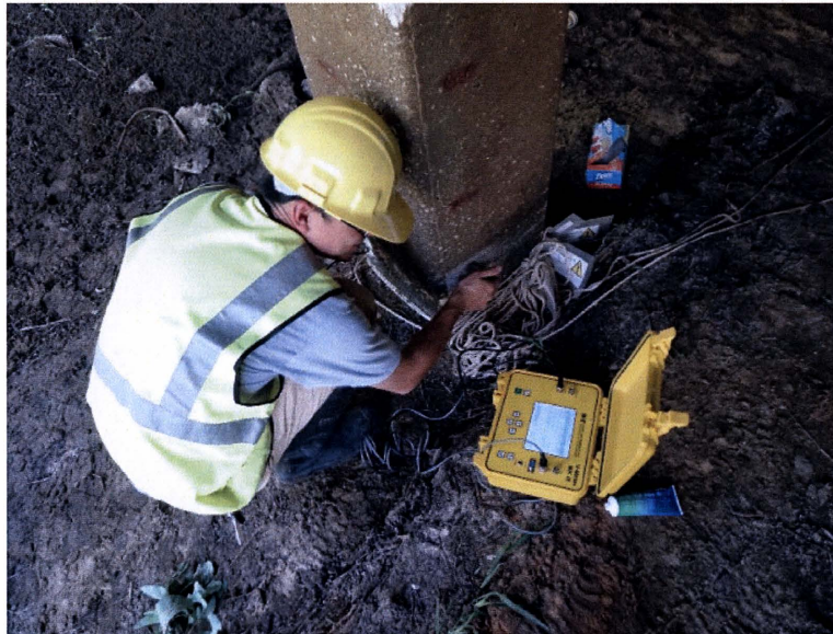
Figure 6 Ultrasonic Pulse Velocity (UPV) Test.
