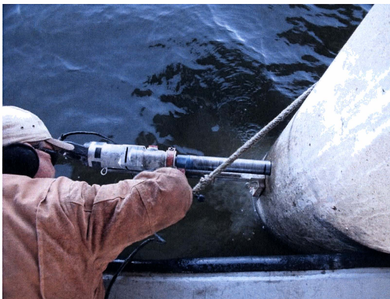
Figure 11. Core Specimen Collection.
