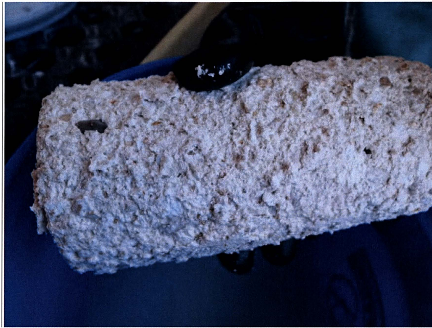
Figure F. 4. Reaction Products on the Surface of Specimen (C-I) after 83 days' Exposure in 3% Sulfuric Solution.
