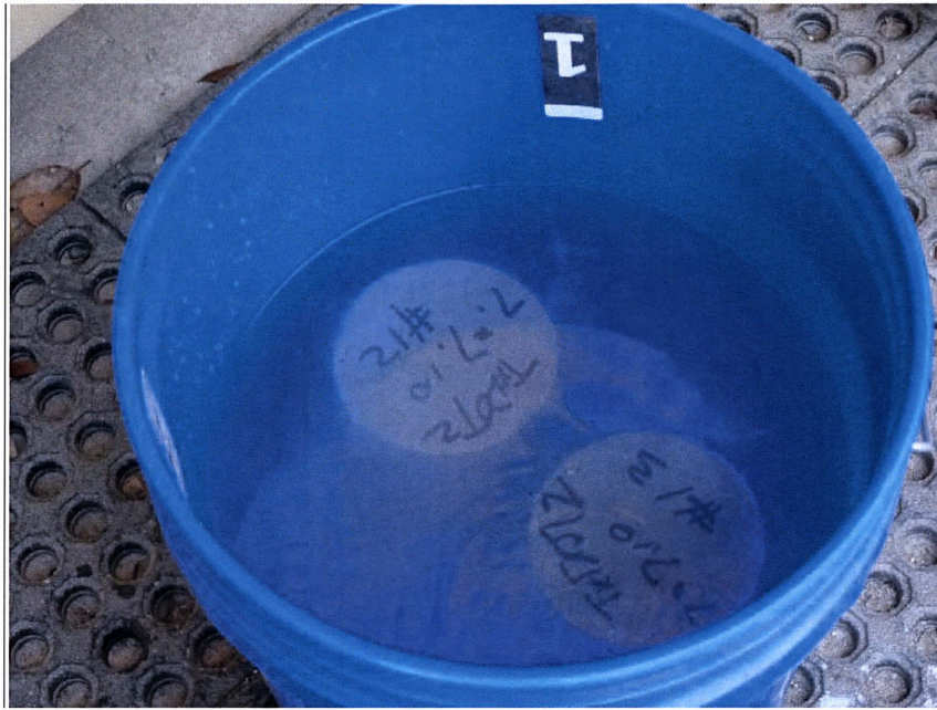
Figure F. 2. Storage of Concrete Specimen in Laboratory Simulation.
