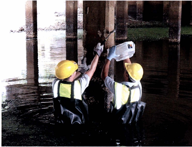
Figure 10. Chemical and Microbial Specimen Collection.
