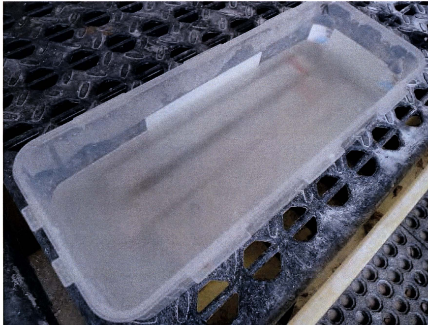
Figure F. 3. Storage of Mortar Specimen in Laboratory Simulation.
