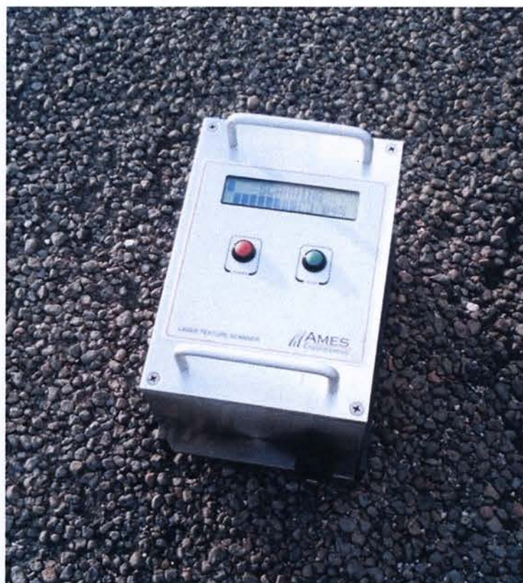
Figure 12. Laser Texture Scanner Taking a Reading.
