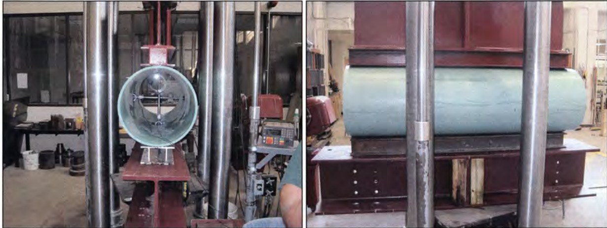
Figure 41. Parallel Plate Loading Test Setup.
