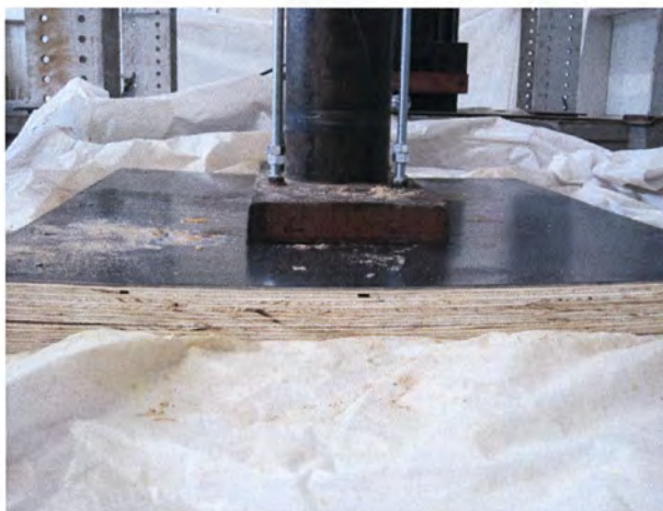
Step 11. Conduct static load test.
