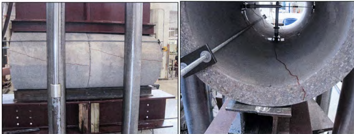
Figure 61. Propagation of Crack of the Jointed Concrete Pipe.
