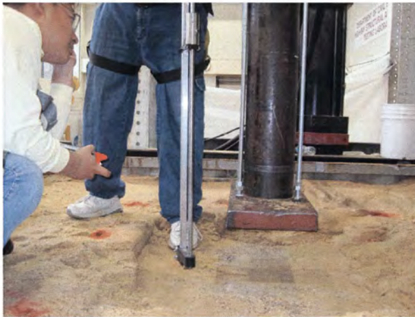
Step 9. Measure backfill soil modulus.
