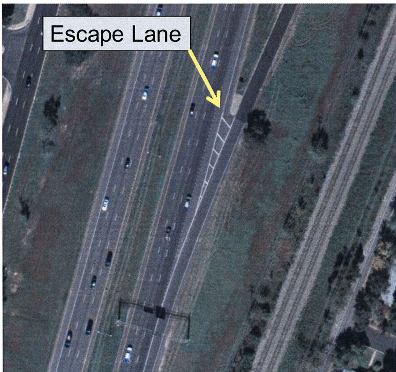
Figure 22. Escape Lanes on Freeway and Exit Ramp.
