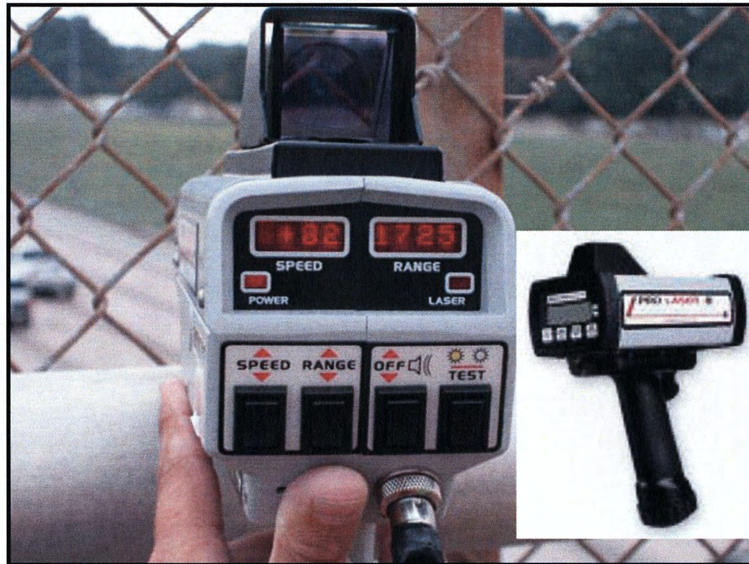
Figure 27. Speed Data Collection Using Lidar (Radar) Gun.
