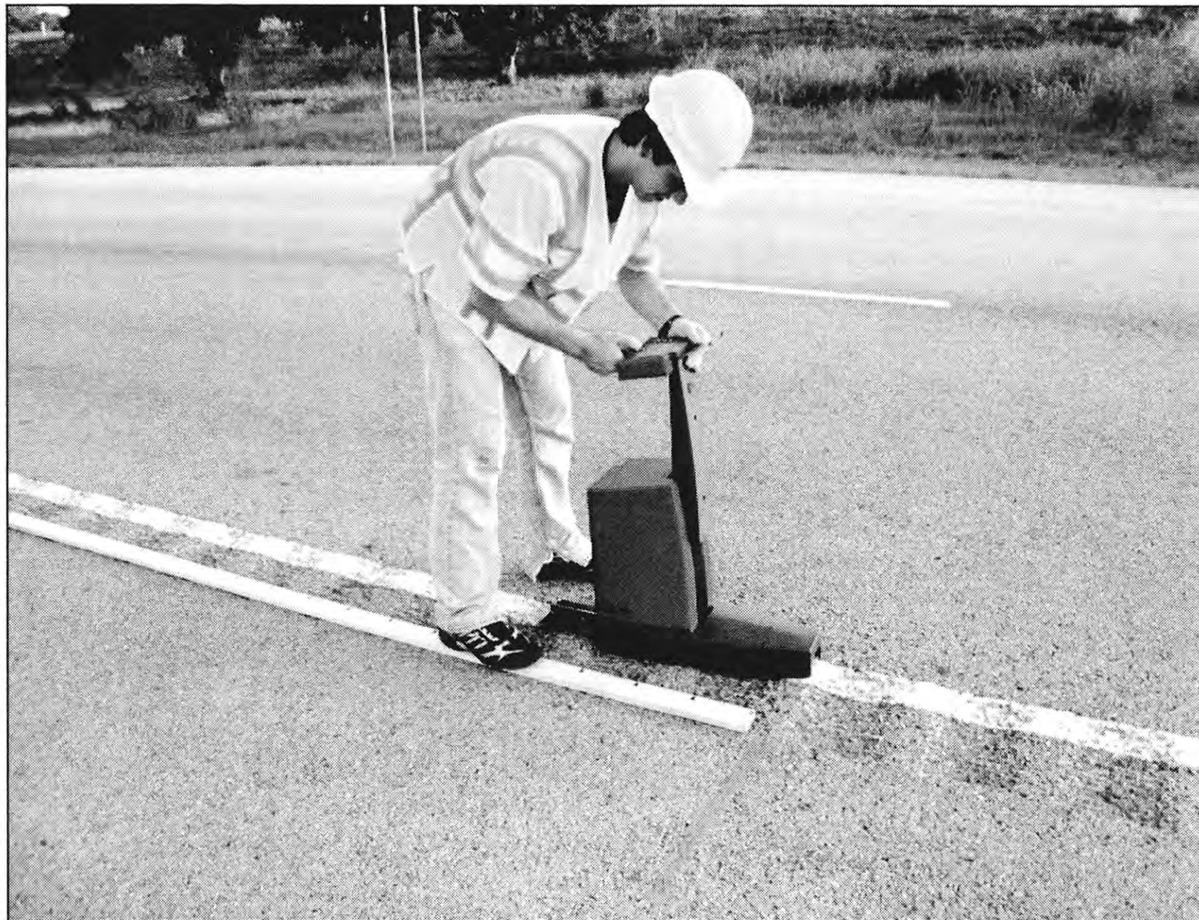
Figure 12. Handheld Retroreflectometer Data Collection on Rumble Stripe.
