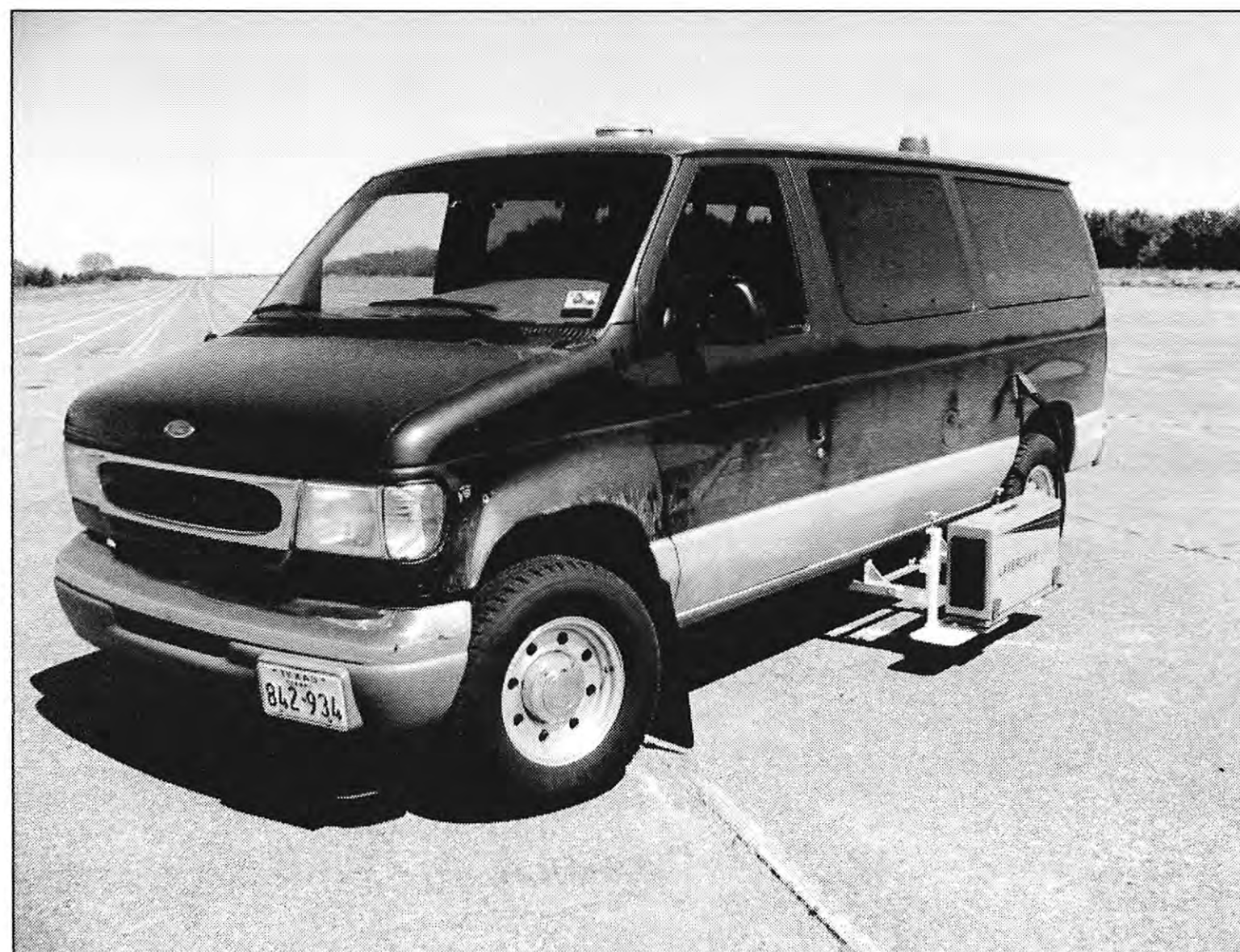
Figure 7. Mobile Retroreflectometer Outfitted on Vehicle.
