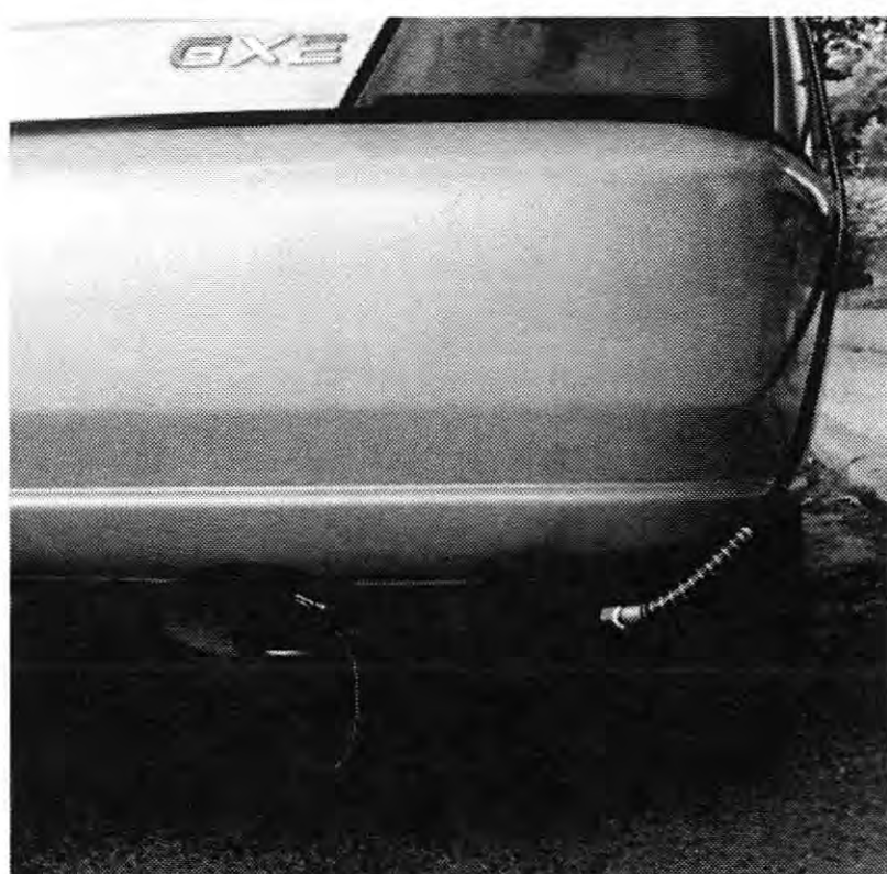
Exhaust Sample Line Secured to the Exhaust System
