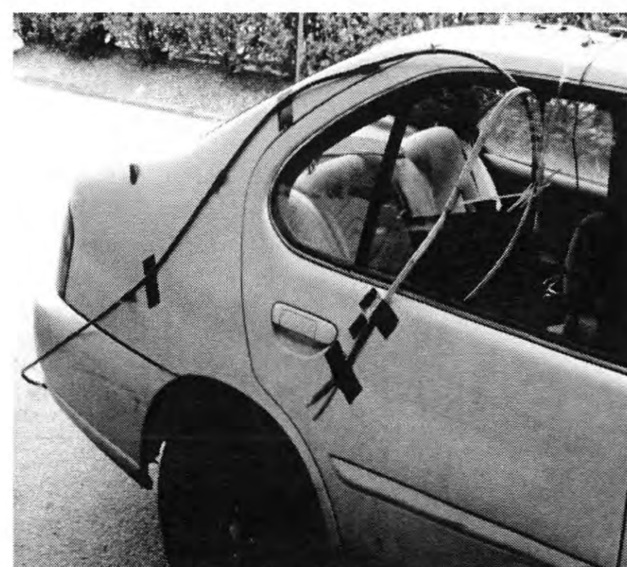
Routing of the Exhaust Sample Lines
