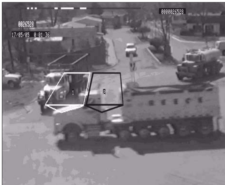
Figure 21. Example Using Traficon Directional Detectors.
