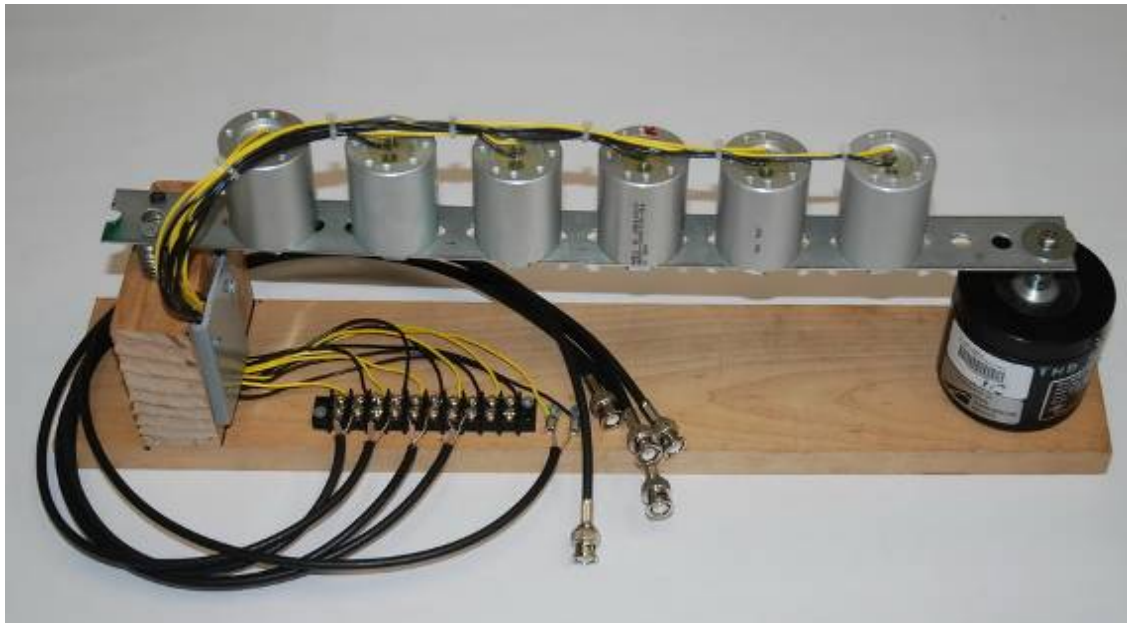
Figure 6.14: TPAD Geophones Simulator Device (Home Made)
