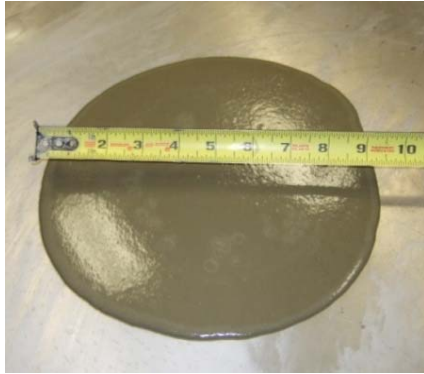
(a) Flow cone displaying good consistency
