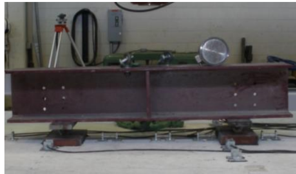
Trailing wheel load over two panels
