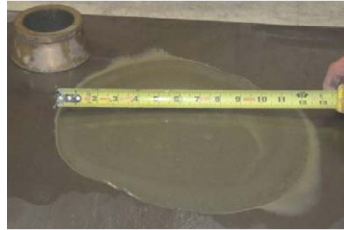
(b) Flow cone showing signs of segregation
