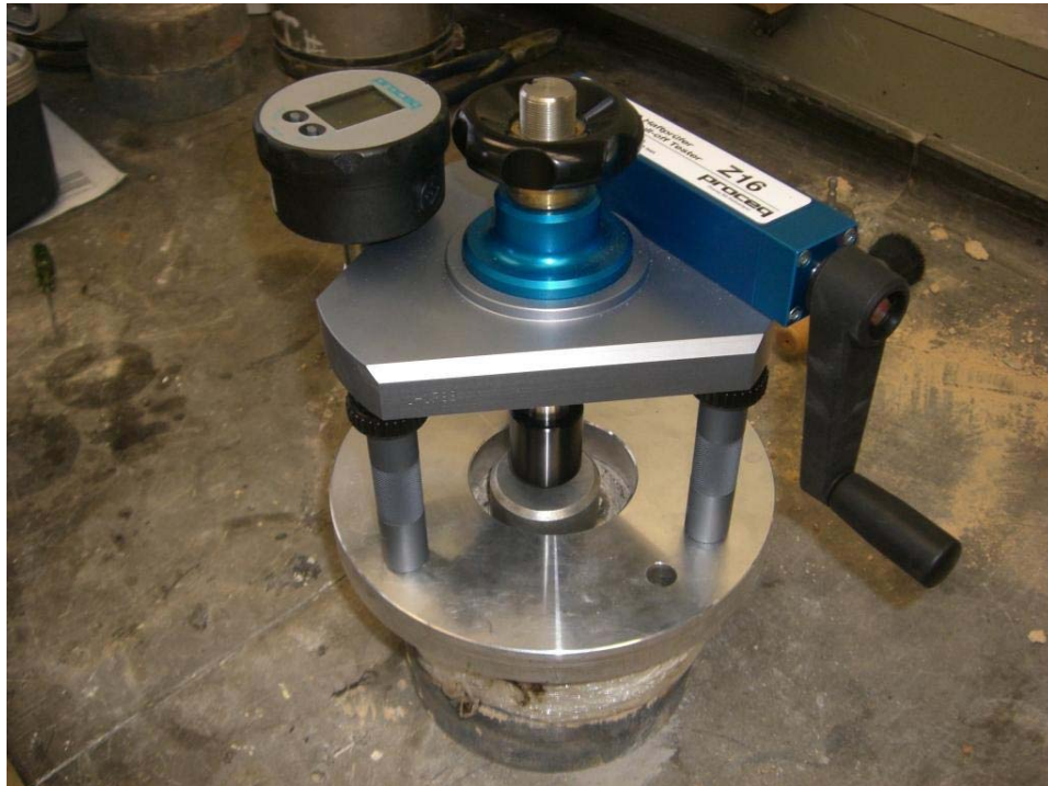
Figure 2.3. Photo of Direct Tensile Bond Test Apparatus.
