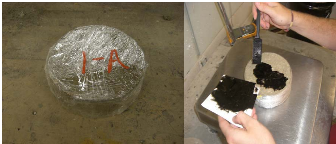
Figure 2.4. Application of Prime to Base Sample.
