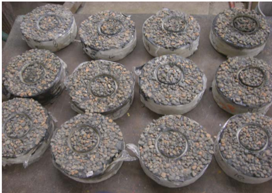
Figure 2.6. Surface Treatment Samples after Coring to a Depth of \frac{1}{2} Inch.
