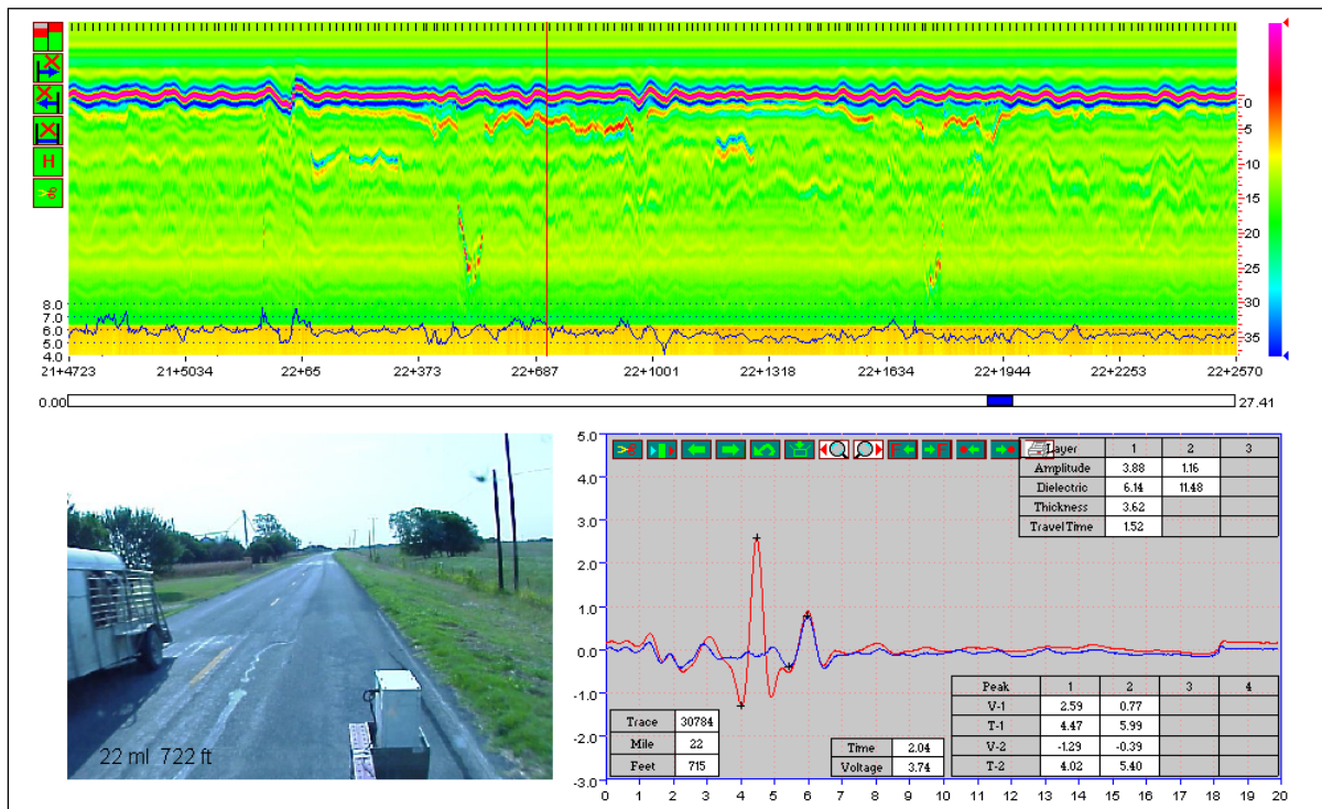
Figure 3.3. Surface Patches and Deep Repairs in GPR Data.
