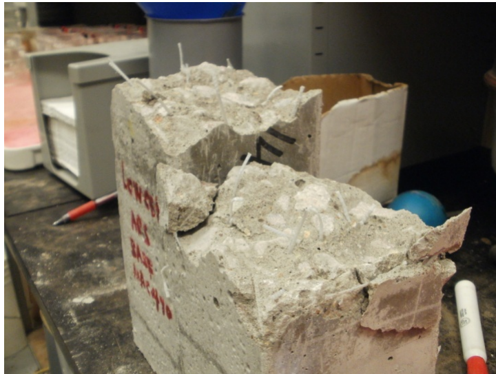
Figure 4.28: Failed interface of the specimen with lowest ARS
