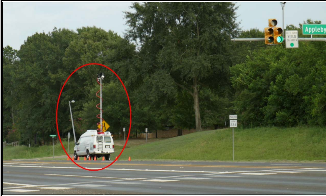
Figure 4-1. Example of Autoscope Van In-Field Setup.
