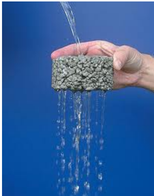
Figure C.9: Pervious concrete (National Ready Mixed Concrete Association 2006)
