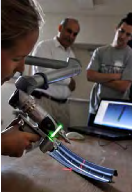
TTI Student Technician Hillary-Anne Metcalfe measures a component using the FARO arm.
