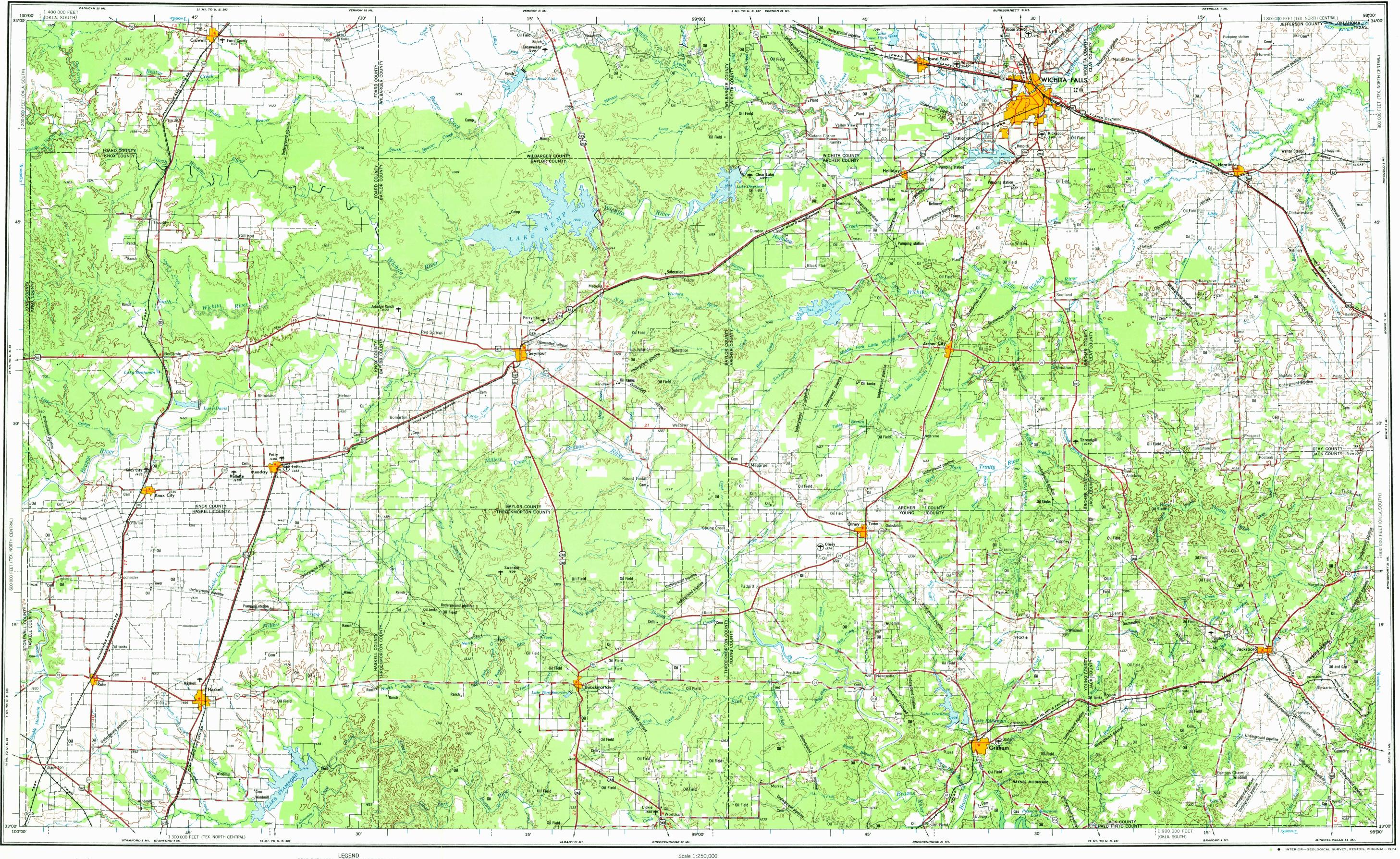
Prepared by the Army Map Service (AJEE), Corps of Engineers, U.S. Army, Washington, D.C. Compiled in 1954 by photogrammetric methods. Horizontal and vertical control by USGS and USC&GS. Aerial photography 1952-1953. Photography field annotated 1954. Limited revision by U.S. Geological Survey 1965.
