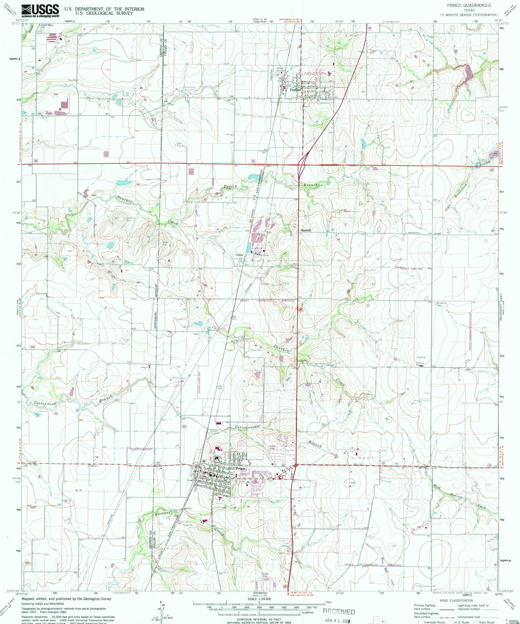
system, north central zone. 1000-meter Universal Transverse Mercator grid ticks, zone 14, shown in blue. 1927 North American Datum To place on the predicted North American Datum 1983 move the projection lines 9 meters south and 26 meters east as shown by dashed corner ticks Fine red dashed lines indicate selected fence and field lines
