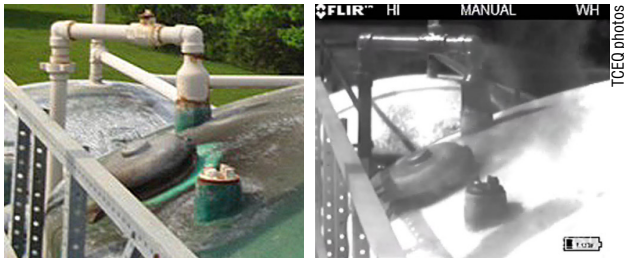
A tank as it looks to the naked eye (left) and the same tank as seen using the IR camera (right). A plume such as this would likely result in further investigation of the site by the TCEQ.
