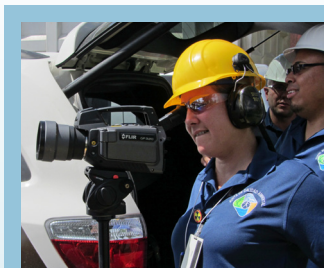
Rebecca Wiscovith, investigator with the Puerto Rico Environmental Quality Board, using the GasFindIR camera to evaluate potential hydrocarbon emissions from an asphalt plant.
