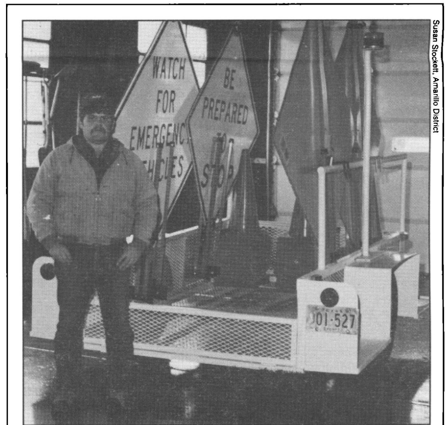
Pete Hare shows off the sign trailer he designed for the Panhandle Maintenance Office, Amarillo District, where he is assistant maintenance supervisor. Fellow employee Jackie Miller built the trailer, used in situations such as emergency lane closures for accidents.
