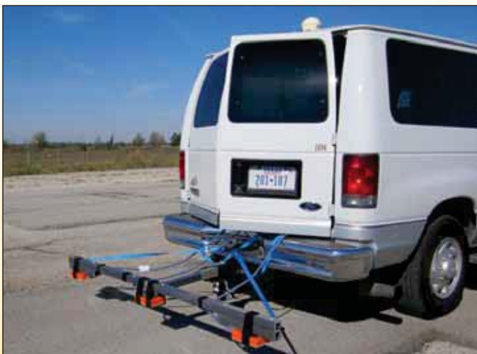
A working prototype of a three-horn 2.6-GHz GPR system designed to be mounted on pickups and vans. This system was tested in November 2012.
