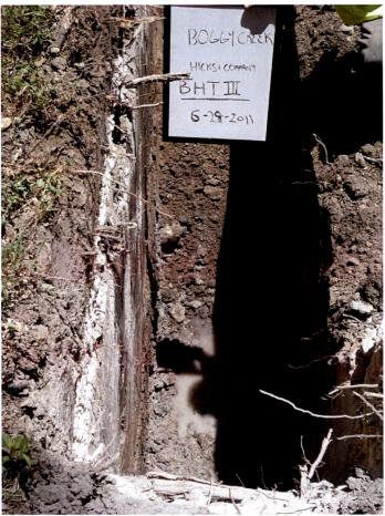
Figure 20: Water table at floor of BHT3.
