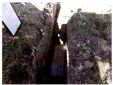
Figure 26: Water table at floor of BHT5.
