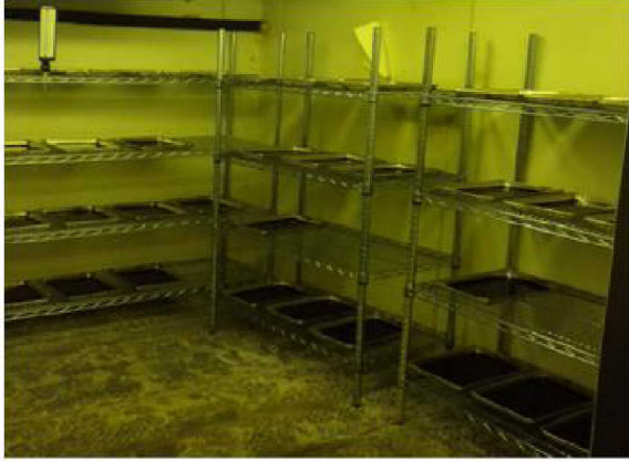
Figure 3.33: Aging of a PG64-22 Control Binder Asphalt samples of 66 grams were poured into trays and allowed to age at the predetermined aging time with a film thickness of 1 mm. Asphalt samples were sampled from the tray for testing after the predetermined aging durations.
