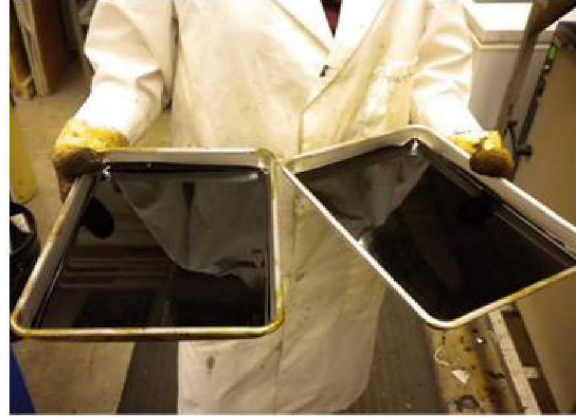
Figure 3.33: Aging of a PG64-22 Control Binder Asphalt samples of 66 grams were poured into trays and allowed to age at the predetermined aging time with a film thickness of 1 mm. Asphalt samples were sampled from the tray for testing after the predetermined aging durations.
