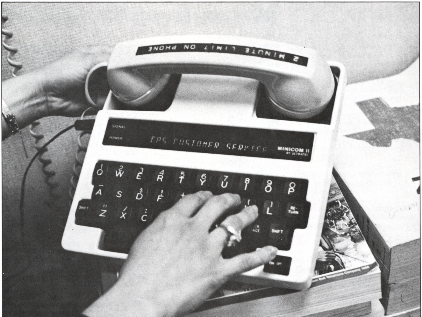
The newly-acquired Telecommunication Device for the Deaf enables hearing-impaired customers to call CPS.
