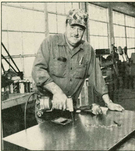
Senior Mechanic Charles Eisenhauer makes a current transformer cover, which protects the device which registers amperes and transfers consumption to meters.
