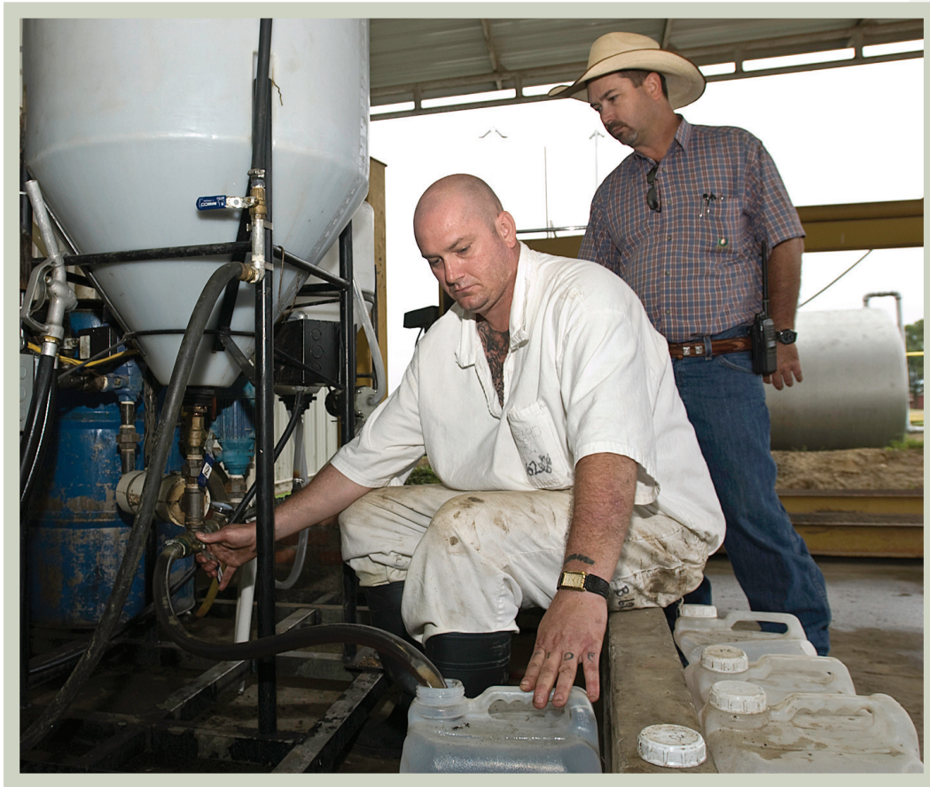
Used cooking oils from TDCJ kitchens are turned into biodiesel fuel for tractors at the Eastham Unit near Lovelady. Here, maintenance supervisor Terry Price (right) watches as pure biodiesel flows from a hose into a plastic container.
