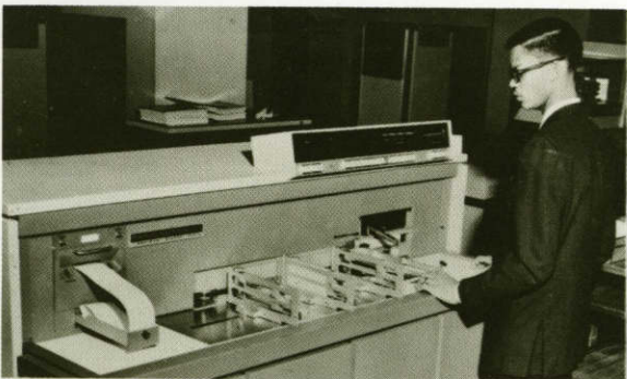
Farrington scanner reads documents at up to 300 per minute.
