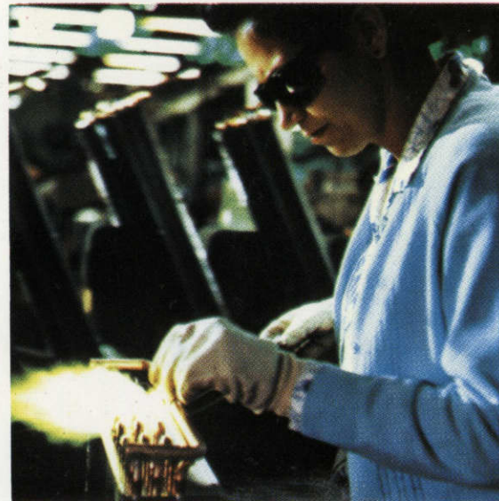
Quality checking coils of air conditioning units
