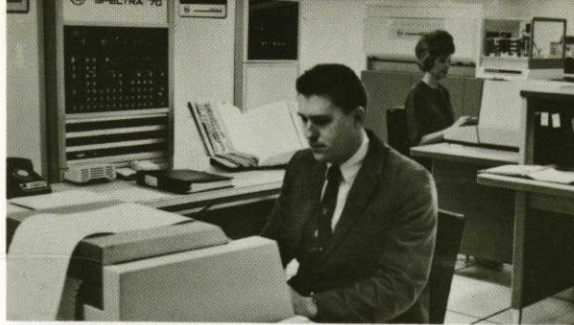
Console in foreground. Left to right, back: central processor, mass storage unit and video data terminal.
