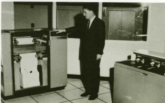
High speed printer has a capability of 1,250 lines per minute.
