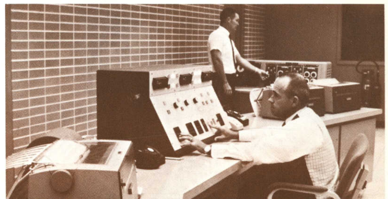
IBM 1800 computer at Braunig Power Plant provides operating data and telemetry.
