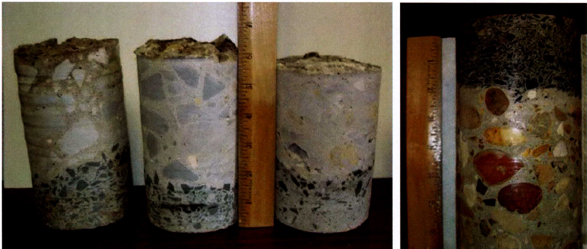
Figure 2. Cross Section of Two-Lift Section in Belknap Place, San Antonio (Ciggelakis et al. 2013; Taylor 2013).
