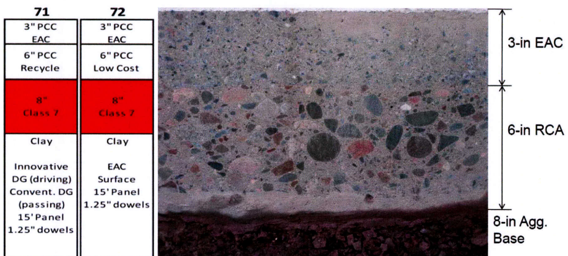
Figure 21. Cross Section of 2LCP Section in Minnesota I-94 Project (Rao and Darter 2011).
