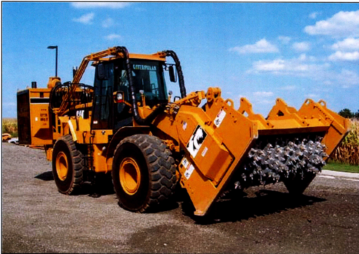
Figure 27. Equipment Used to Mix Soil with Lime.
