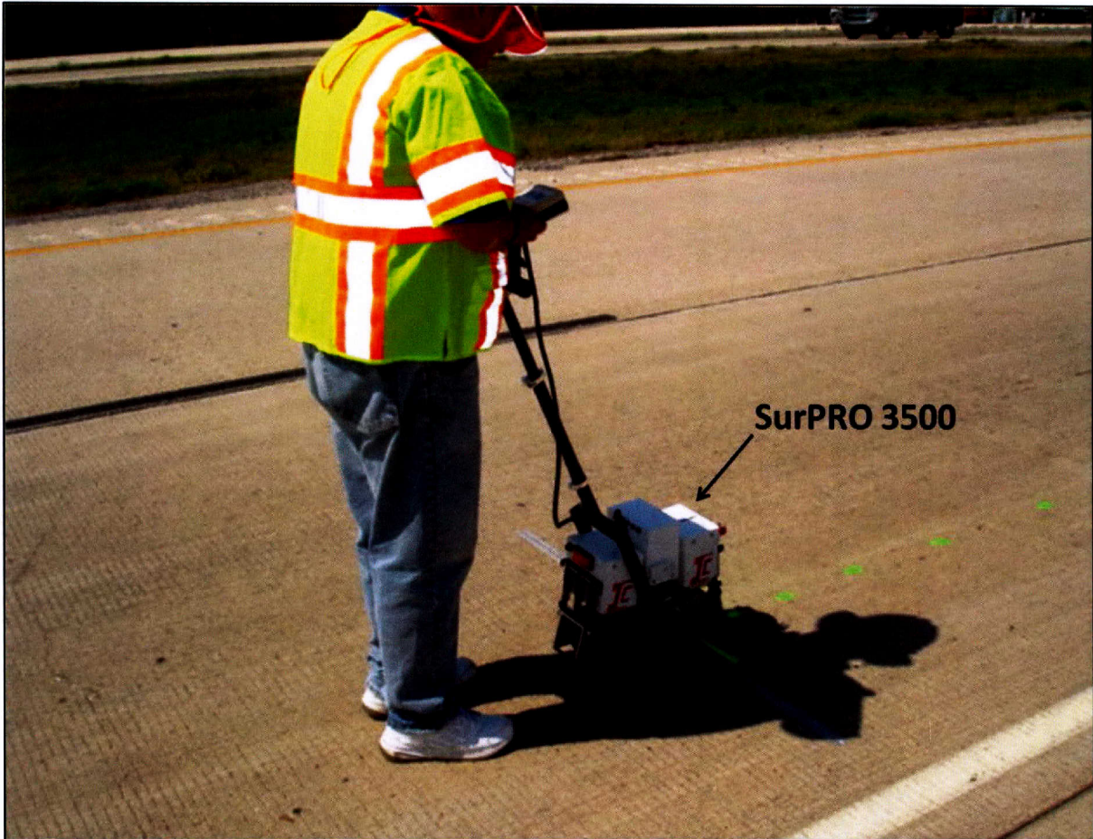
Figure 57. Instrument Used to Measure Reference Profiles.
