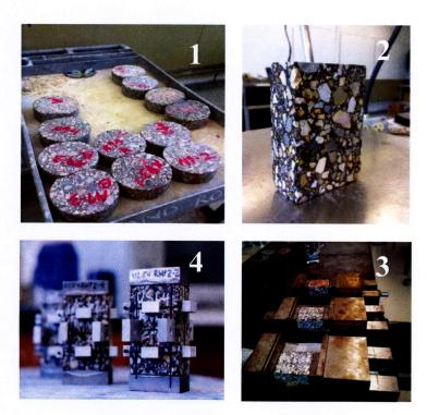
Figure 42. Sample Preparation for VEC Test.
