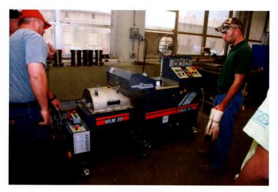
Figure 1. Wirtgen Laboratory Scale Foamed Bitumen Equipment in TTI's Laboratory.
