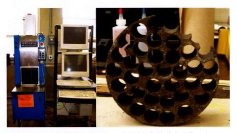
Figure 102. SGC Compactor and DMA Cylindrical Specimen.
