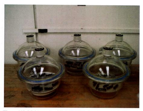
Figure 103. Moisture-Conditioned DMA Specimens in Desiccators.
