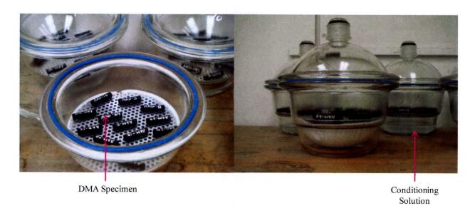
Figure 104. DMA Specimens Conditioning in Desiccators.
