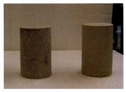
(a) Fresh Cylindrical Limestone Specimens Cored from Limestone Rocks
