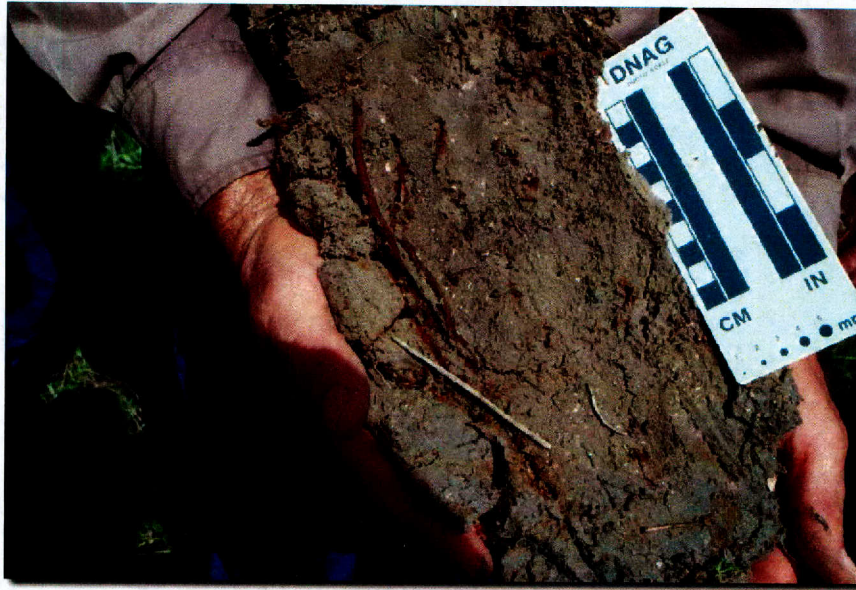
Figure 5.7. Redoximorphic concentrations of iron (red zones) along root channels are a strong indicator that this soil undergoes prolonged periods of saturation and reduction. Photo J Jacob
