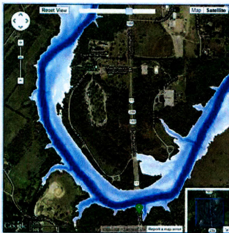
C) Largest flow recommended by the Guadalupe-San Antonio BBASC; 14,000 cfs with an elevation of roughly 123.9' (NAVD88).
