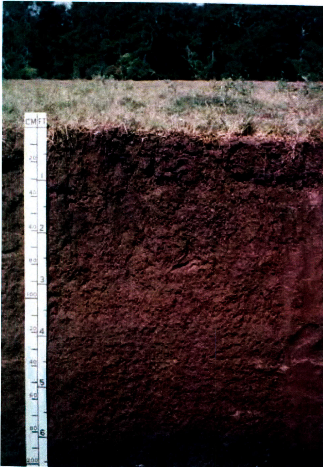
Figure 5.20. Profile of Brazoria Clay, taken from the pdf manuscript of the Colorado County soil survey. The profile is clayey throughout. Note the presence of a buried A horizon at about 6.5 feet.
