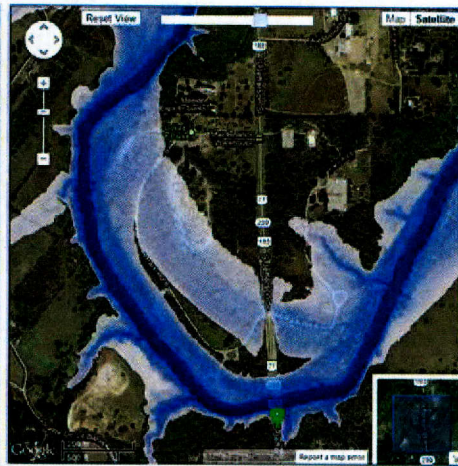
B) Largest flow recommended by the Guadalupe-San Antonio BBEST; 23,600 cfs with an elevation of roughly 130.9' (NAVD88).
